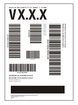
Figure 40 • FEED Test Label
